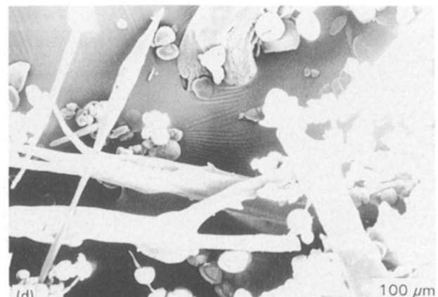
Figure 7 Scanning electron micrographs of the LCP phase in various PP/LCP blends after dissolving the PP matrix. (a) PP/9% LCP; (b) PP/17% LCP; (c) PP/29% LCP; (d) PP/33% LCP and (e) another area of the same PP/33% LCP specimen.
