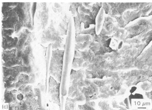
Figure 5 Scanning electron micrographs of the fracture surfaces of (a) PP/9% LCP, (b) PP/17% LCP and (c) PP/29% LCP, after being chopped parallel to the flow direction at liquid-nitrogen temperature.
